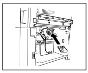
**10** If finisher F-8430 is installed, close right-side door FN7.
